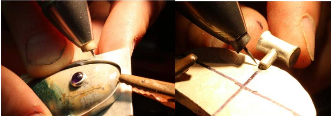
**Tack Welding Multiple Parts Together Before Soldering Using Small Amounts of Glue onto Sheet Metal Connected to a Positive Electrical Lead.**
